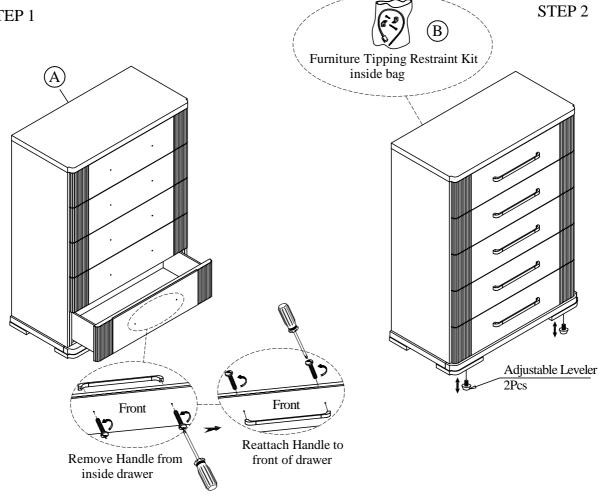
For product and personal safety, a Furniture Tipping Restraint kit has been included with this unit which can help to minimize the risk of the unit accidentally tipping forward, if used and properly installed per the kit manufacturer's instructions.
